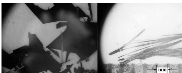
Fig. 6 Platelet-shaped crystals of (\text{NEt}_4)[\text{Pd}(\text{dmit})_2]_2 (left) and fiber-shaped crystals of “ (\text{PrNEt}_3)[\text{Pd}(\text{dmit})_2]_2 ” (right). (\text{Me}_3\text{NEt})[\text{Pd}(\text{dmit})_2]_2 and (\text{MeNEt}_4)[\text{Pd}(\text{dmit})_2]_2 have the same crystalline habits as (\text{NEt}_4)[\text{Pd}(\text{dmit})_2]_2 .
